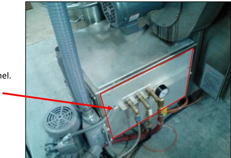
3) Using a 5/32" Allen wrench remove the screws that hold on the side, and top panels, and remove them.
