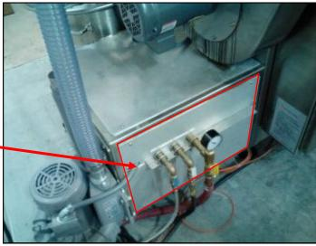
3) Using a 5/32" Allen wrench remove the screws that hold on the side, and top panels, and remove them.
